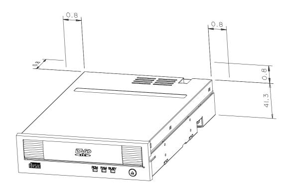
• Do not apply force (under 1.5N: 150gf) caving in the top plate.
